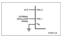
Figure 5. External Clock Drive Configuration
