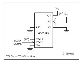
Figure 8. I<sub>CC</sub> Test Condition Idle Mode. All other pins disconnected.
