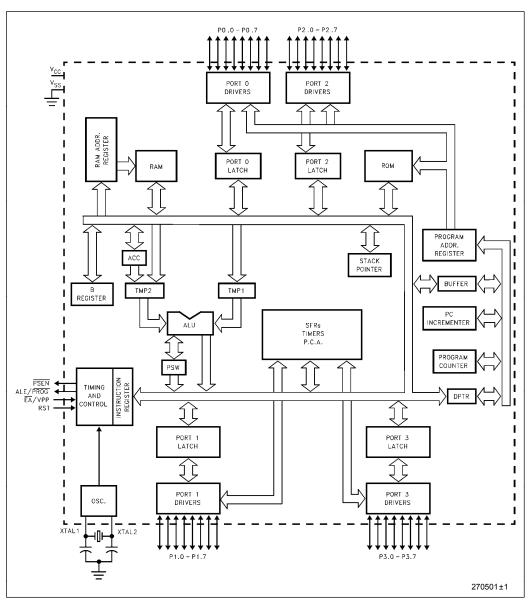
Figure 1.83C51FA Block Diagram
