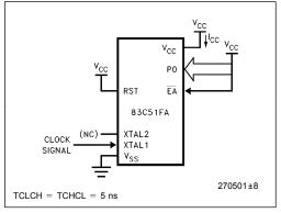
Figure 7. I<sub>CC</sub> Test Condition, Active Mode All other pins disconnected.
