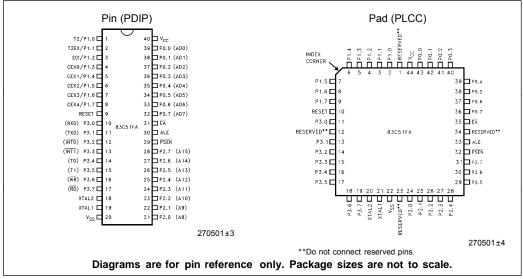
Figure 3. Pin Connections
