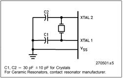
Figure 4. Oscillator Connections
